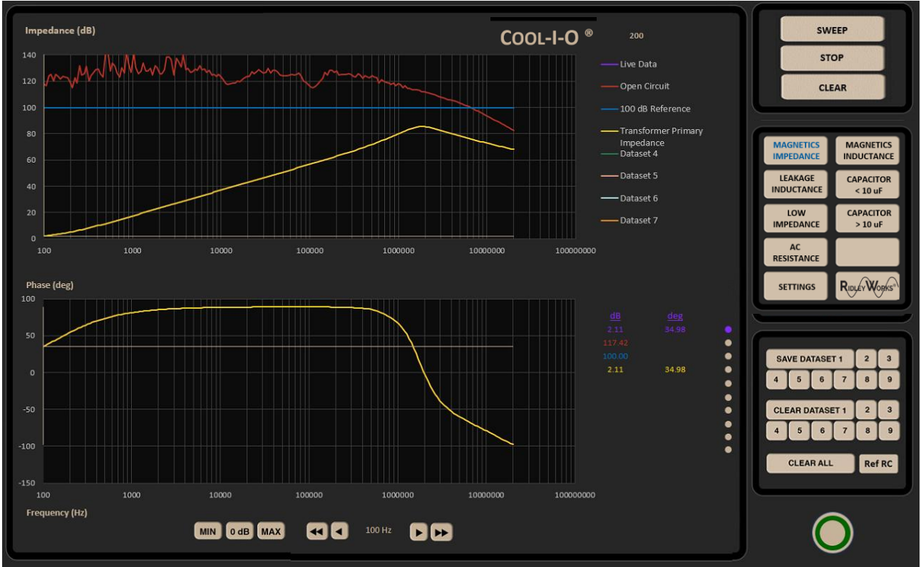
Fig. 4.2: Impedance Dynamic Range and Transformer Measurement
